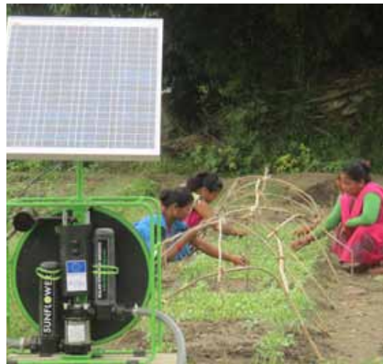
Solar lift (Sunflower Pump) Irrigation
